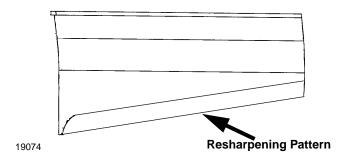
Do not sharpen to original pattern (below). It is easier to get a straight cutting edge following the resharpening pattern shown above.
